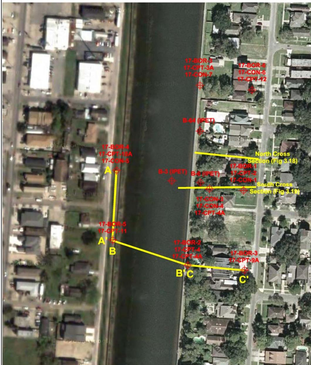
Figure 3.17: Aerial photo of the 17<sup>th</sup> Street Canal breach site before the failure of August 29, 2005. The yellow lines (at middle right) indicate the positions of the geologic sections presented in Figures 3.17 and 3.18, while cross sections A-C' are shown in Figure 3.21.
